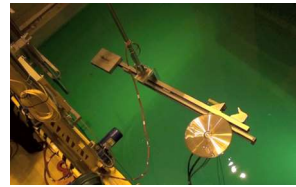
Equipment for Internals Segmentation At Jose Cabrera
