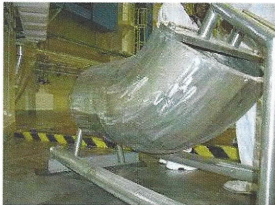
Figure 35: Primary loop piping mock up made purposely for NDT calibration/validation which was used for real efficiency calibration at Slovak NPP Bohunice.
